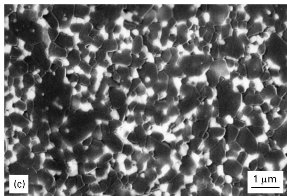
Figure 6 Scanning electron micrographs of sintered (2 h at 1550 °C), polished and thermally etched RBAO samples. (a) A/C, (b) B/C and (c) B/C contaminated by the addition of 0.3 wt % calcined kaolin.
